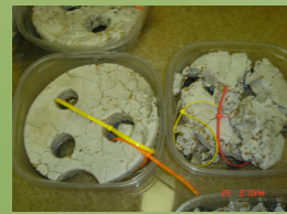
Figure 4: Fert-Discs in laboratory testing environment. Note structural integrity of cement fortified (left) vs. unfortified (right) plaster
