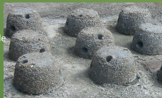
Figure 2: Armored cultivator units awaiting deployment. (photo: J. Krumholz)
