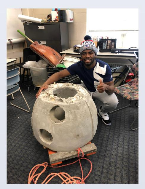
Figure 1: Each Min-Bay Ball RBM weighs 90kg and provides  $2.9m^2$  of surface area and was constructed using materials and guidelines provided by the Reef Ball Foundation.
