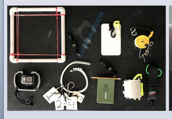
Figure 7: Pictured above is all the materials needed for *Method 2*. This Figure 8: Photo taken on 3/28/2019 of diver 1 measuring the length of the includes; 1 Quadrat, 1 Ruler with 4 paper clips attached, 1 Write in the rain living oysters on RBM1 Quadrat A while diver 2 takes photos and hold booklet, 1 GoPro in a waterproof casing, 5 zip ties with numbers attached, 1 quadrat steady. retractable spool to attach diving flag to, 1 pair of shears, and 2 dive slates.
