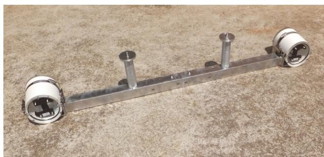
*Fig 8. Stereo-Video analysis software and camera bar (SeaGis Australia) used in the accurate measurement of fish lengths for biomass calculations.*
