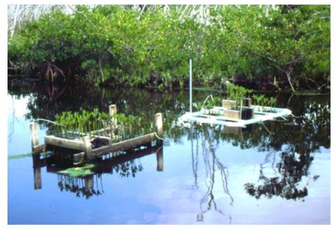
Fig. 3. In the field experiments, fixed and floating nurseries of planted red mangrove seedlings were monitored for plant growth and survival in controlled impoundments and open bay sites.
