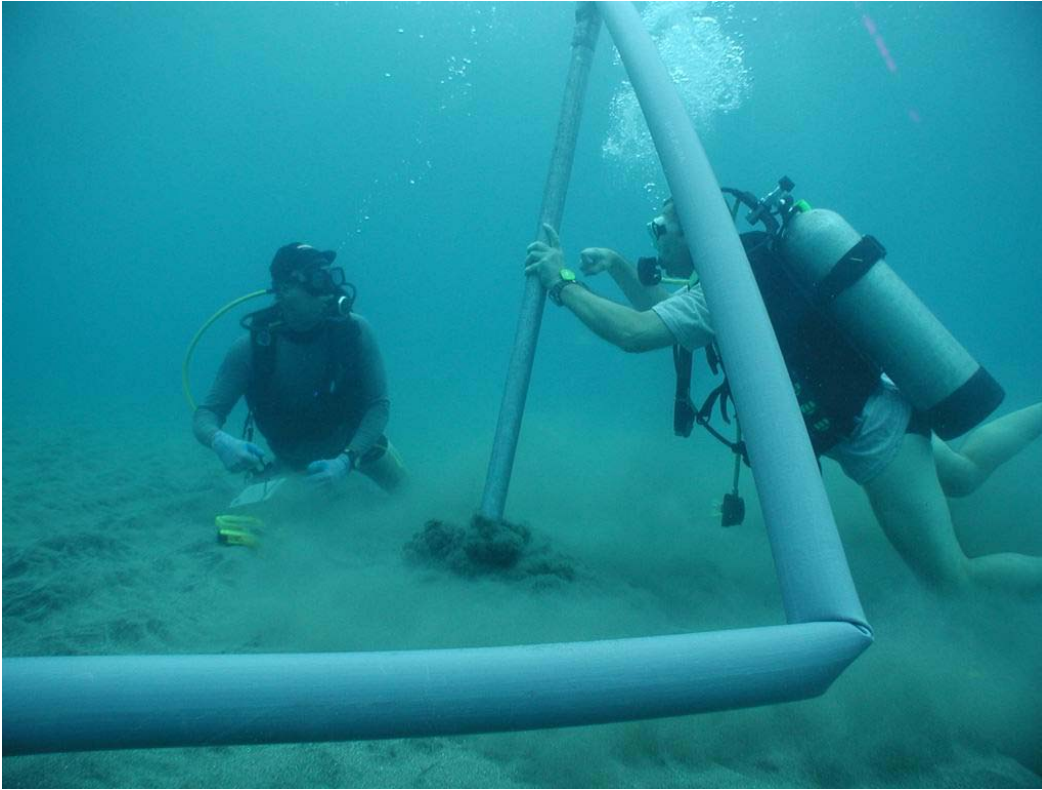
Figure 13. Water Jet Probes being Performed
