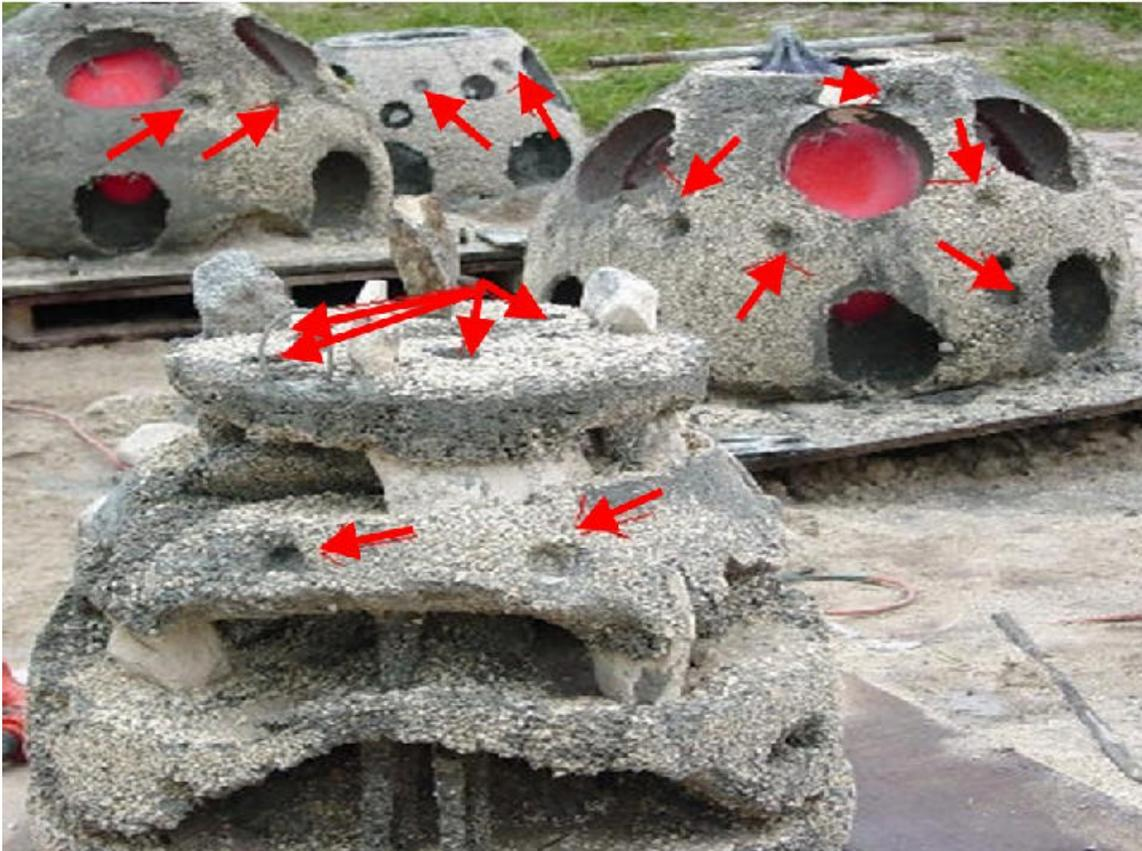
Figure 10: Different styles of Reef ball artificial reef modules equipped with coral plug adapters indicated with red arrows.
