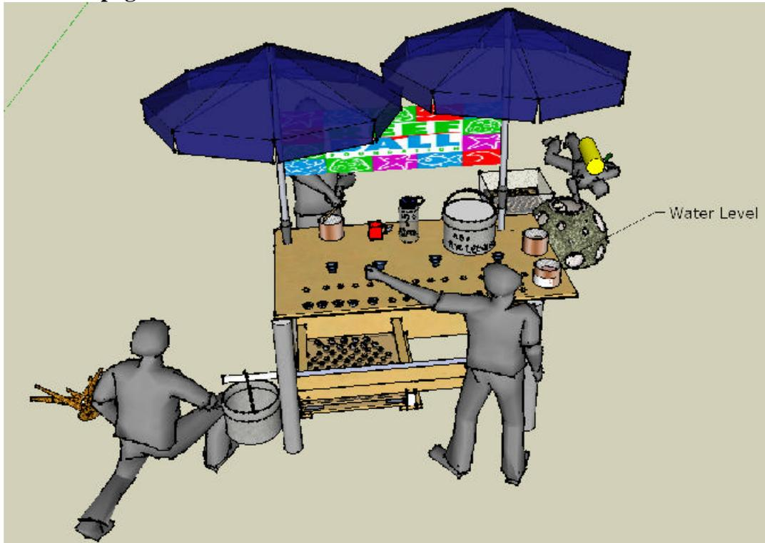
Figure G16: Beach based coral table (available in Sketch-Up™). Table must be underwater to the point where the coral planting tray is under water at all times, and protected from heavy surge. Umbrellas shade the entire table from sunlight. Coral table workers from left to right, 'wet hands' (kneeling), table boss (behind table), dry hands.
