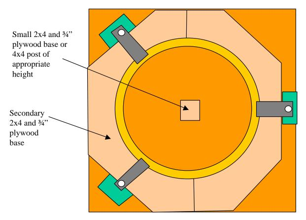
Plan view of Mini-Bay Ball mold system with two-piece flange cover for pouring concrete flanges
