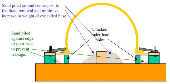
Cross section of mold with center pedestal or 4x4 post for positioning Polyform buoy
