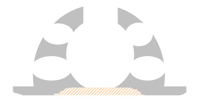
Cross section of Mini-Bay Ball with integrated cast anti-settlement/stability flanges. Crosshatched area, when not filled in with concrete, used to provide anti-slide friction in lieu of bottom waves created using sand during pour.
