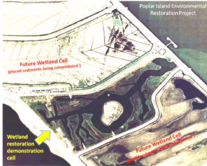
Figure 1 Initial wetland demonstration cell at Poplar Island Environmental Restoration Project. Fully functional marsh and intertidal habitat inside an armored sand dike enclosure. Culverts with a sufficient cross section relative to circulation needed enables unrestricted natural tidal conditions but precludes access by watercraft.
